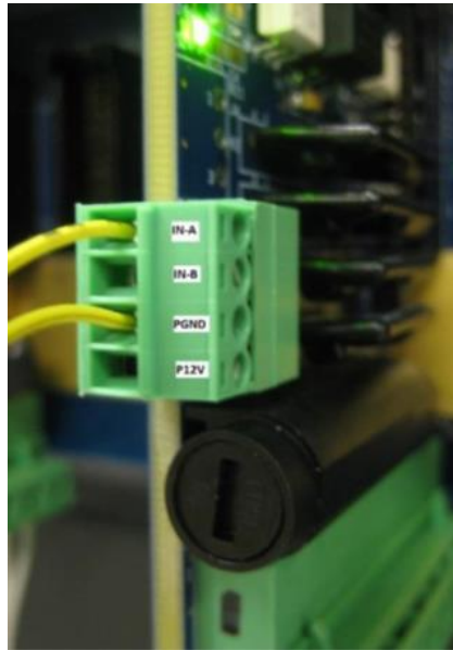
Figure 17 – Minimal Pulsar Connector Wiring for a mechanical pulsar
